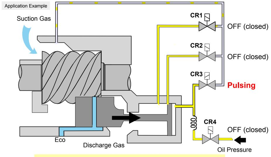
position between 50% .. 25% – less capacity required
