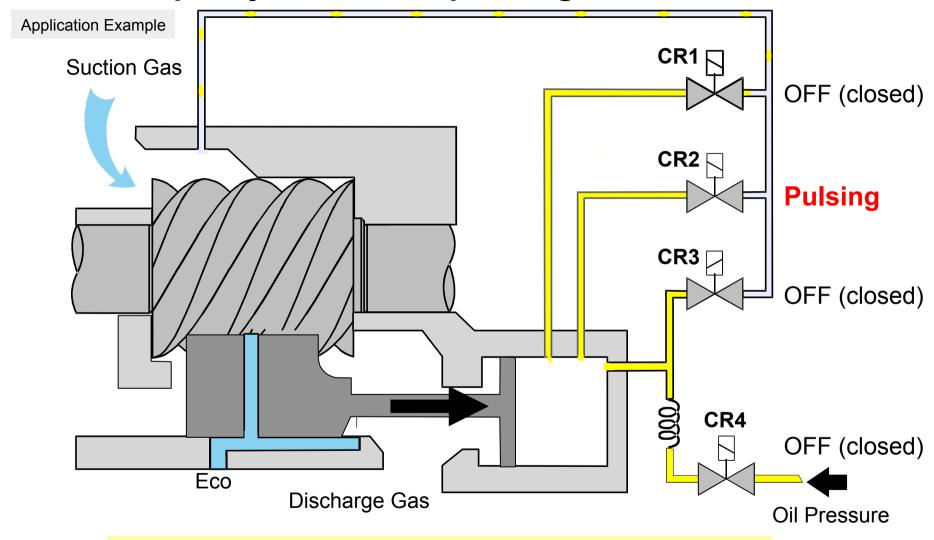
position between 100% .. 75% – less capacity required
